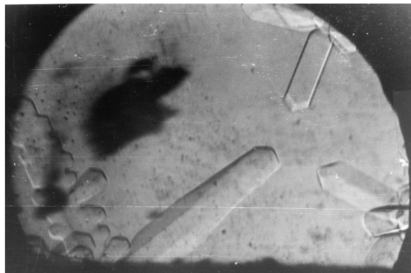
FIG. 36 . ^3\text{He} crystals growing at 80 mK (Rolley et al. , 1986). The facets are the (110) surfaces.
