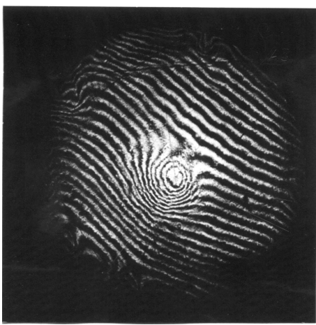
FIG. 16 . Interference pattern of a charged liquid-solid ^4\text{He} interface (Bodensohn et al. , 1986). The field of vision is about 2 cm in diameter. Here the electrons are concentrated in the central region to enhance the visibility of the deformation. The parallel fringe pattern outside the center results from a small angle between the two interferometer plates.
