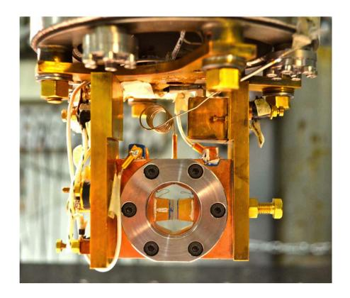
FIG. 2. The experimental cell that was used to measure the mechanical properties of <sup>4</sup>He crystals at ENS in 2013-2014. Single crystals are grown from the bottom up inside the 0.7 mm slit between two vertical transducers in the center of the cell. The crystal orientation was obtained from photographs of the growth shape in the bottom part.
