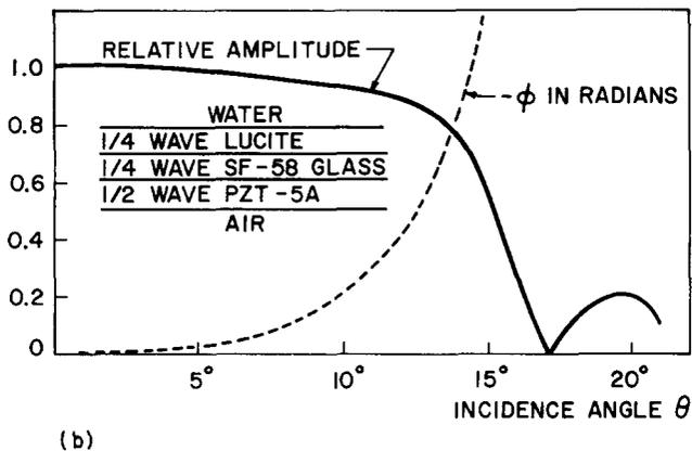
FIG. 2. Angular response of (a) unmatched, and (b) matched PZT transducers. Stiffened velocities and impedances are used.
