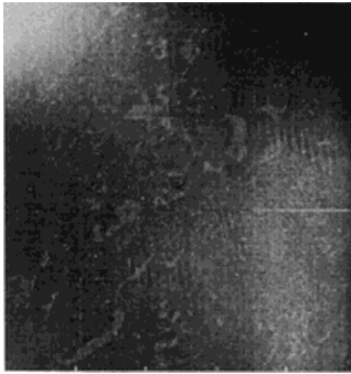
Figure 8. AFM images of a monolayer of PCA deposited on silicon at a pressure < 0.1 mN/m and a molecular area of 0.7 nm 2 . The image is 100 × 100 μm 2 .
