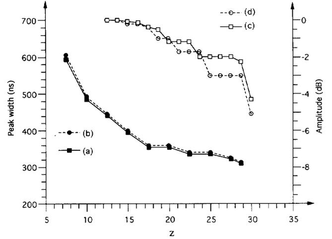
Fig. 4. Diffraction filter effects. Variation of the peak amplitude (c, d) and variation of the peak width at  $-20$  dB (a, b) versus the normalized distance  $Z$  for  $m$ -sequence (continuous lines) and Golay's codes (dotted lines).
