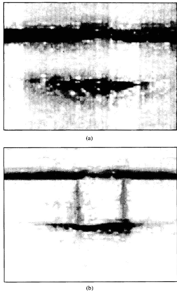
Fig. 9. Echo B type image of a single hole drilled in AGA14 (dural). (a) Pulse method. The bottom of the hole is clearly visible. (b) Correlation with *m*-sequence. The bottom and the side walls of the hole are visible. Hole dimensions: diameter = 3 mm, depth = 10 mm.
