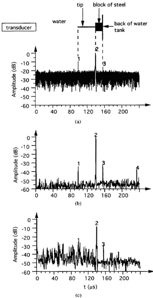
Fig. 8. The object and the corresponding echograms as obtained with (a) classical pulse method, (b) *m*-sequence, (c) complementary series.
