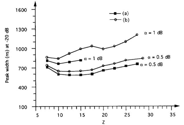
Fig. 5. Same as Fig. 4 but the effects of attenuation are added ( $\alpha = 0.5$  dB or 1 dB) (a) 1023 bit  $m$ -sequence; (b) two 1024 bit Golay's codes.
