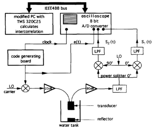
Fig. 7. Schematic representation of the digital correlation system assembled in our laboratory. LO: Local oscillator, LPF: Low-pass filter,  $e(t)$ ,  $S_1(t)$  and  $S_2(t)$  are, respectively, the reference code, the two received signals applied to the correlator.
