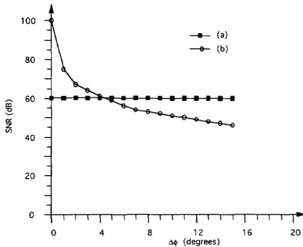
Fig. 6. SNR degradation versus phase error  $\Delta\phi$  between two 1024 bit Golay's codes. A variation of  $10^\circ$  in  $\Delta\phi$  induces a SNR of 40 dB (this corresponds to  $\Delta d = \frac{\lambda\Delta\phi}{2\pi} = 120 \mu\text{m}$ ).
