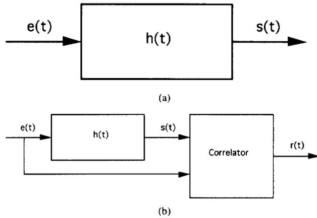
Fig. 1. Schematic block diagram of the ultrasonic imaging system. (a) Classical system. (b) System using correlation techniques.
