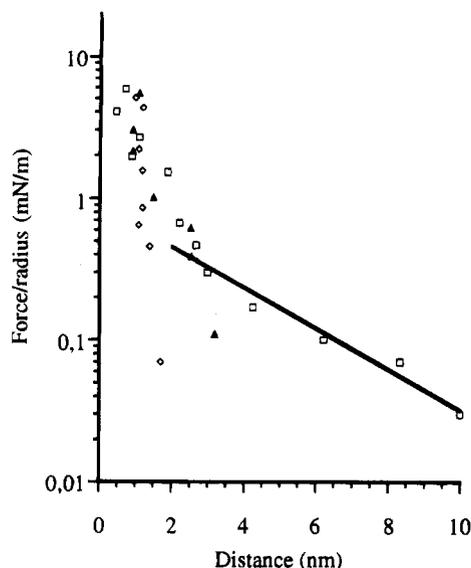
**Figure 4.** Normalized force versus separation distance between a deposited film of cellulose acetate (on mica) and mica in  $10^{-2}$  M KCl solution at pH 2 (open diamonds), pH 5 (filled triangles), and pH 11 (open squares). The distance is that between the compressed cellulose acetate film and mica. The line is the theoretical Debye decay length (3 nm). Only decompression results are shown.
