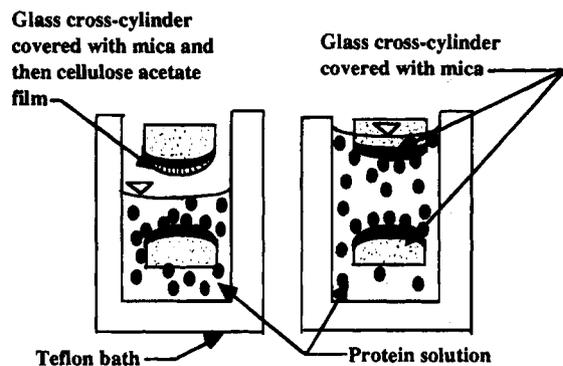
**Figure 2.** Schematic showing the two cross-mica cylinders for (a) one surface covered with the protein solution and for (b) both surfaces covered with the protein. In part a this ensured that protein was not adsorbed onto the upper surface.
