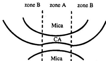
**Figure 8.** Hypothetical diagram of the compaction of cellulose acetate film in the SFA.
