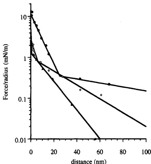
**Figure 6.** Normalized force versus separation distance between a deposited film of cellulose acetate and an adsorbed human serum albumin protein layer in a  $10^{-2}$  M KCl solution at pH 2 (filled circles), pH 4.8 (open diamonds), and pH 9 (filled triangles). The full lines represent the curves obtained with the values given in Table 2. The distance was that between the precompact cellulose acetate film and a compressed layer of human serum albumin. Only decompression is shown.
