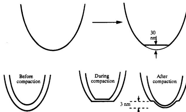
**Figure 9.** Surface deformation due to glue during compaction of the cellulose acetate film.
