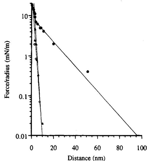
**Figure 7.** Normalized force versus separation distance between a deposited film of cellulose acetate and an adsorbed ribonuclease A protein layer in a  $10^{-2}$  M KCl solution at pH 5 (filled circles), pH 9.2 (open diamonds), and pH 11 (filled triangles). The full lines are from fits to the data with the values given in Table 3. The distance was that between the precompact cellulose acetate film and a compressed layer of ribonuclease A. Only decompression is shown.
