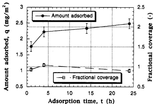
**Figure 1.** Amount of hydrated RNase A adsorbed and fractional surface coverage on mica as a function of time. The solution contained a RNase A concentration of 0.1 mg/mL in  $10^{-2}$  M KCl, pH 5, and at  $20 \pm 0.5$  °C.
