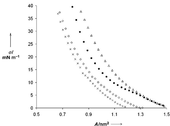
**Figure 2.** Isotherm compression measurements of lipid monolayers at an air/water interface.  $\sigma$  is the surface tension and  $A$  is the molecular area; pure SOPC (x), 1:9 SOPC/CerLLe<sup>x</sup> (or CerLLe<sup>a</sup>) mixture (◇), pure Le<sup>x</sup> neoglycolipid (△),<sup>[11]</sup> and pure CerLLe<sup>x</sup> or CerLLe<sup>a</sup> (●).
