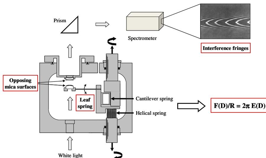
FIGURE 1. The Surface Force Apparatus (SFA).
