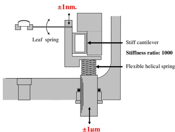
FIGURE 2. The differential spring system.
