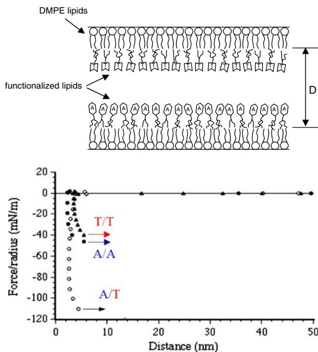
**FIGURE 4.** Interaction between DNA bases measured by SFA. The mica surfaces are coated with bilayers functionalized to carry nucleosides on their lipid headgroups. The adhesion measured in the complementary system (A/T) is much larger than for the symmetrical systems (A/A and T/T).
