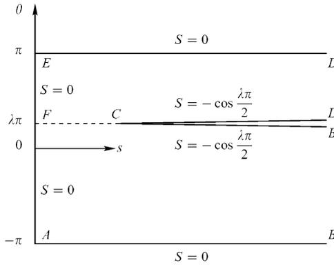
Fig. 2. The  $(s, \theta)$ -plane, with  $s \geq 0$  and  $-\pi \leq \theta \leq \pi$ , that maps the region III of  $(r, \theta, t)$ -space, corresponding to  $r \leq ct$ ,  $-\pi \leq \theta \leq \pi$ , and  $t > 0$  (see Fig. 1).
