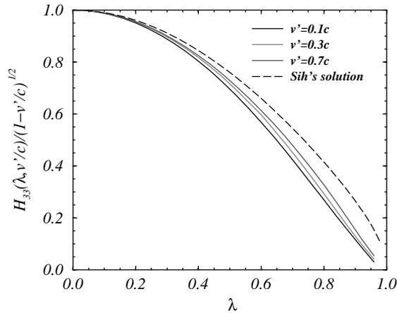
Fig. 5. Plot of the stress intensity factor function  $H_{33}$  as a function of the kinking angle and for different values of the crack tip velocity. Also shown in this figure, Sih's solution associated with the elasto-static kinking problem (Sih, 1965).
