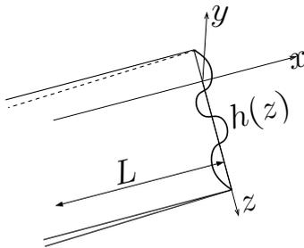
**Fig. 1** –. Schematic of the problem of a half-plane crack on  $y = 0$  in an infinite body. The average penetration of the crack front in the  $x$ -direction is  $L$ . The straight reference front in the  $z$ -direction and the perturbation  $h(z)$  around it are also shown.
