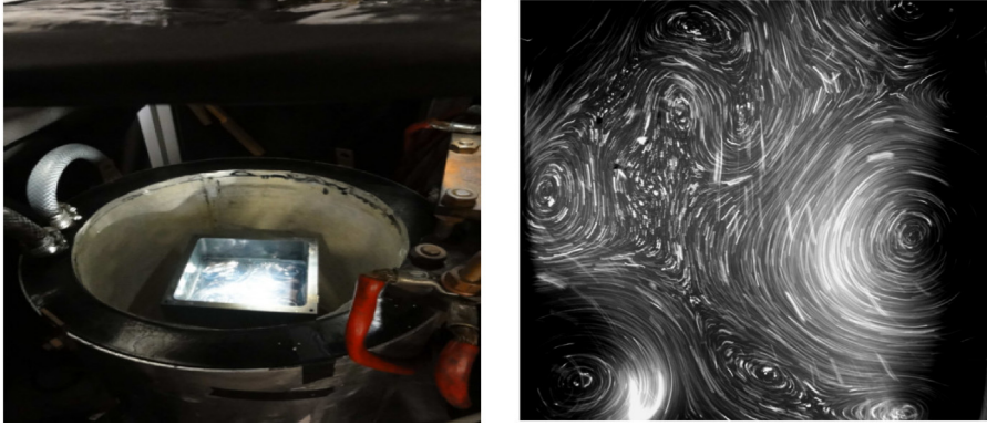
Fig. 60. Left panel: View of an experimental set-up to study liquid metal flows in the quasi-static limit. Right panel: Visualization by tracer particles of the resulting large-scale vortex in the presence of an inverse cascade. The images provided by J. Herault display the experimental apparatus used in the works [393–395].
