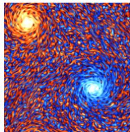
Energy condensation in 2D turbulence
