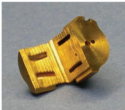
**Figure 1** | Strong evidence. The 'strong' beryllium-copper cell used by West *et al.*<sup>5</sup> to demonstrate that supersolidity exists in solid helium-4, but not in solid helium-3. The cell has been cut to show the free annular space inside, which is filled with helium at low temperature and high pressure. The diameter of this annular space is 1 cm. Image courtesy of Joshua West.
