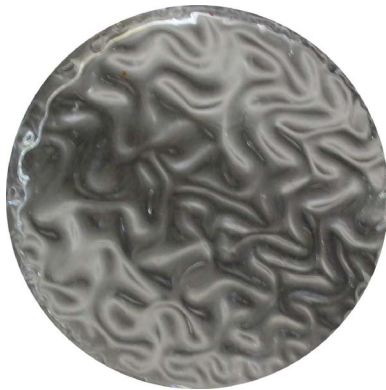
Fig. 1 Top view after swelling of the top layer (thickness h = 1 mm above a 3 cm thick substrate) in a dish of 10 cm diameter. The valleys are lighter than the crests. The lighting is not uniform as a dark strip was placed below to increase the contrast.
