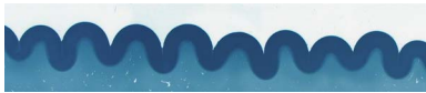
Fig. 4 Side view of the gel top layer (colored with ink) after swelling. Thickness h = 3 mm (after swelling), wavelength \lambda = 8.9 mm, and amplitude A = 5.1 mm.
