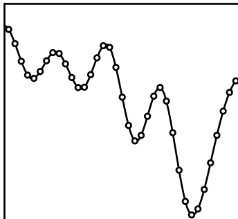
Figure 2.5: Rugged energy “landscape” which poses problems in a dynamical Monte Carlo simulation at low temperatures. The system will be stuck in one of the local minima, and the dynamics will be futile, i. e. very repetitive.
