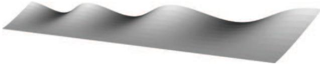
**Fig. 4.** Most unstable mode for an infinite flat strip of gel longitudinally compressed on one edge, as given by the solution to equation (8).
